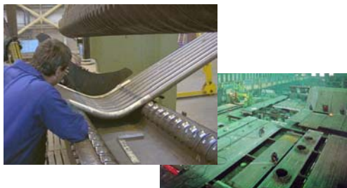
Test bending furnace wall panels in T23 material
