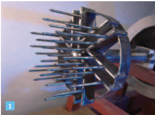
1: Temperature Monitoring System for Nuclear Boiler Header
